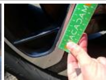
Tyre FR, Out of tolerance, Replace
