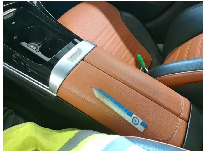
Damage 3: Instrument panel: Centre console - front - Broken / torn - Smart repair
