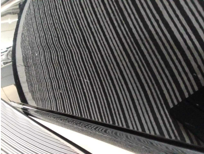
Damage 5: Door - front right side: Door - Defective - Smooth repair work
