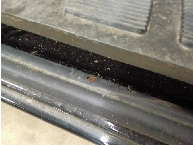
Damage 8: Sliding door, right: Door seal - Broken / torn - Replace
