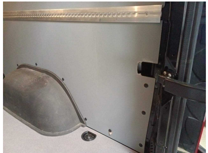
Damage 10: Side panel - rear right side: Interior trim - Broken / torn - Replace
