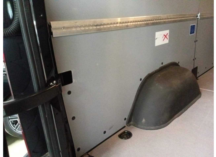
Damage 9: Side panel - rear left side: Interior trim - Broken / torn - Replace
