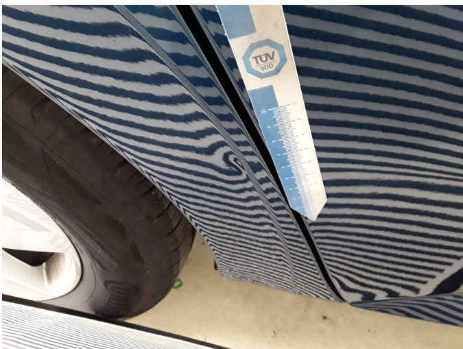
Damage 3: Side panel - rear right side: Side panel - dent(s) - Smart repair
