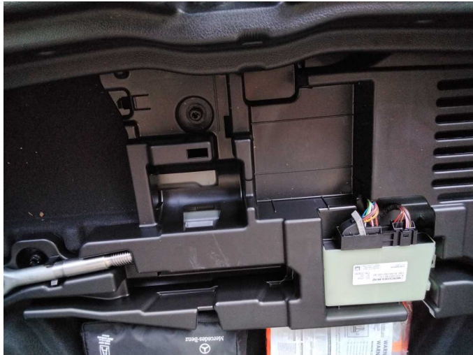
Missing part 1: Equipment: Tirefit complete - Missing - Replace
