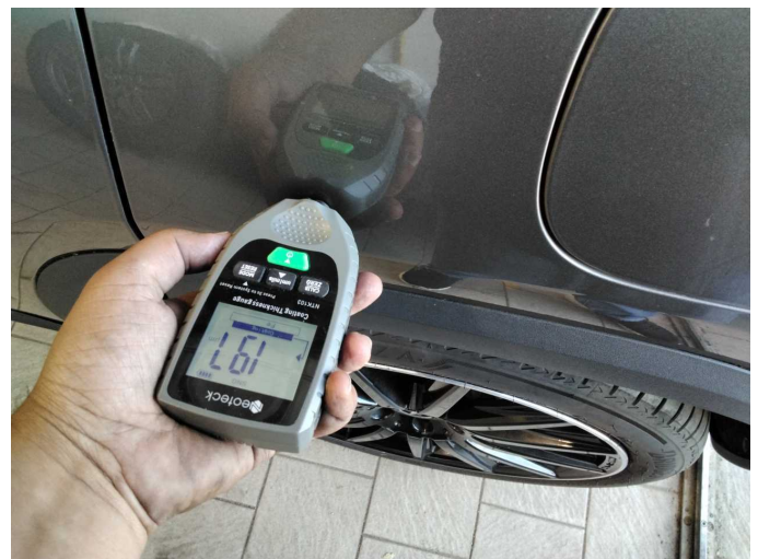
Side panel - rear left side: 197 µm
