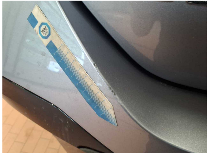
Damage 10: Rear bumper: Rear bumper - Scratch(es) - Paint
