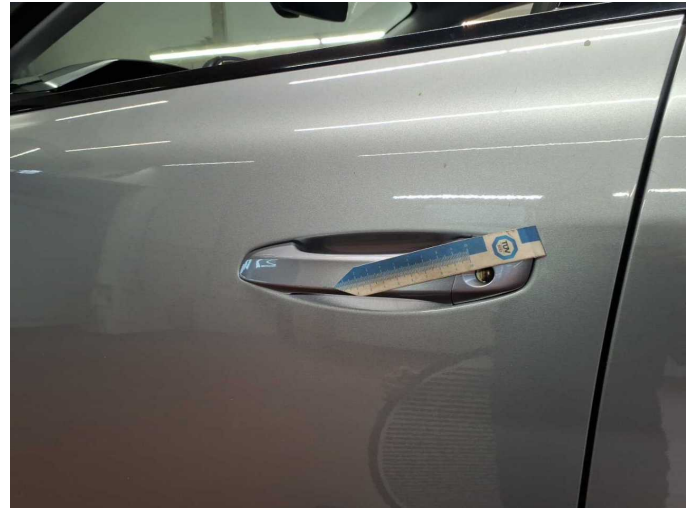
Damage 1: Door - front left side: Door handle - outside - Scratch(es) - Smart repair
