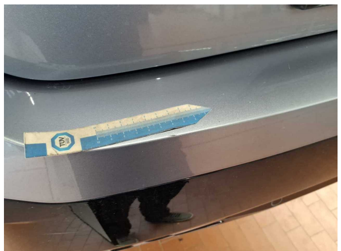
Damage 10: Rear bumper: Rear bumper - Scratch(es) - Paint
