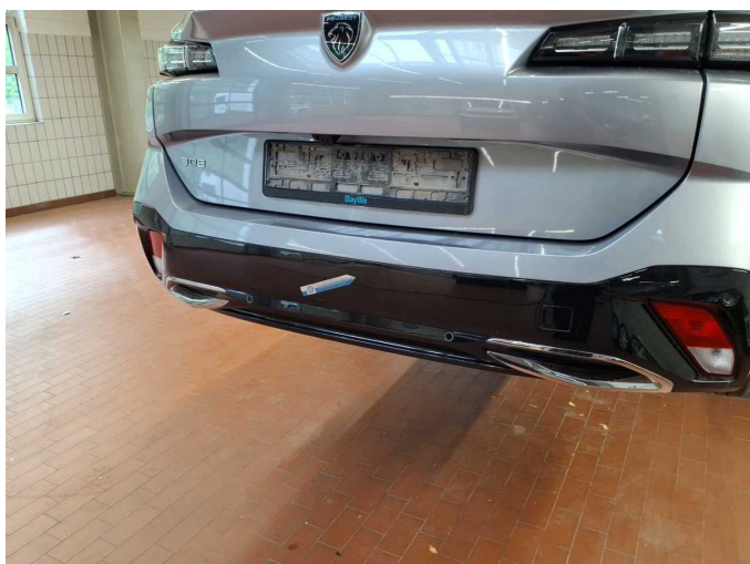
Damage 9: Rear bumper: Spoiler - Dent / paintcoat damage - Replace
