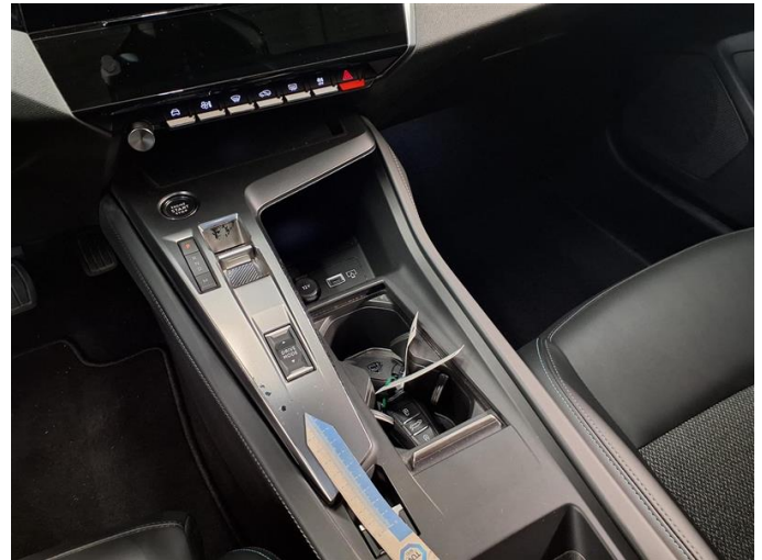
Damage 6: Instrument panel: Centre console - front - Porous / cracked - Replace
