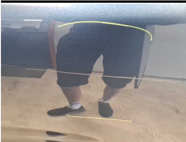
Damage #5: Door - rear left side: Door - Scratched - Repair and paint
