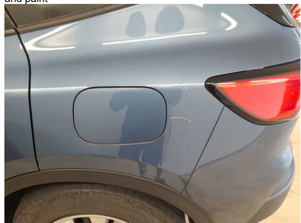
Damage #7: Side panel - rear left side: Side panel - Scratch(...) - Repair and paint
