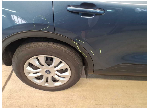
Damage #4: Side panel - rear right side: Wheel well extensio... Scatched - Replace
