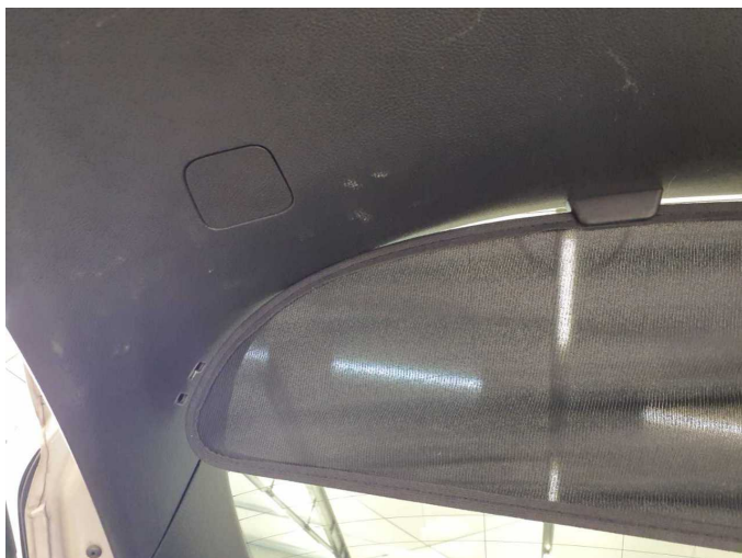
Damage 1: Interior: Roller blind rear window (Halterung) - Missing - Replace
