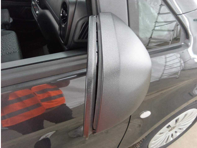
Damage 3: Wing mirror - right side: Cap - Malposition - Un- / install
