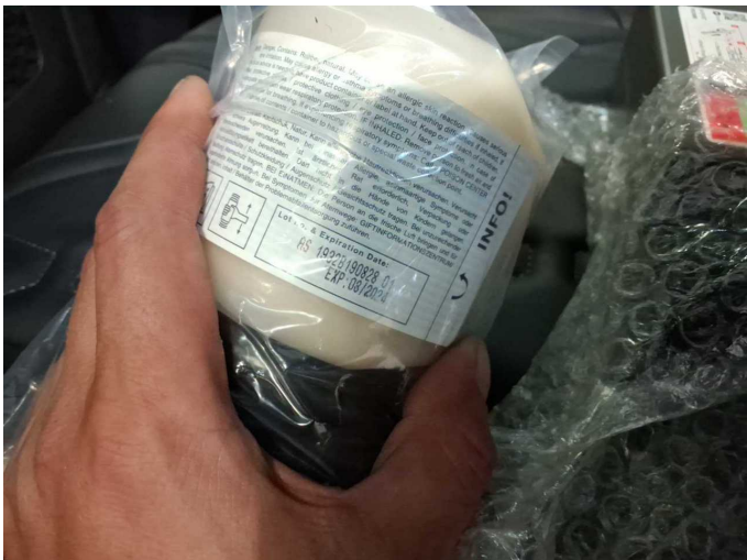
Damage 1: Equipment: Tirefit filler - Expired - Replace
