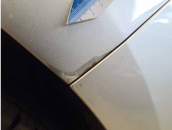
Damage 5: Side panel - rear left side: Side panel - Unprofessionally repaired - Repair and paint
