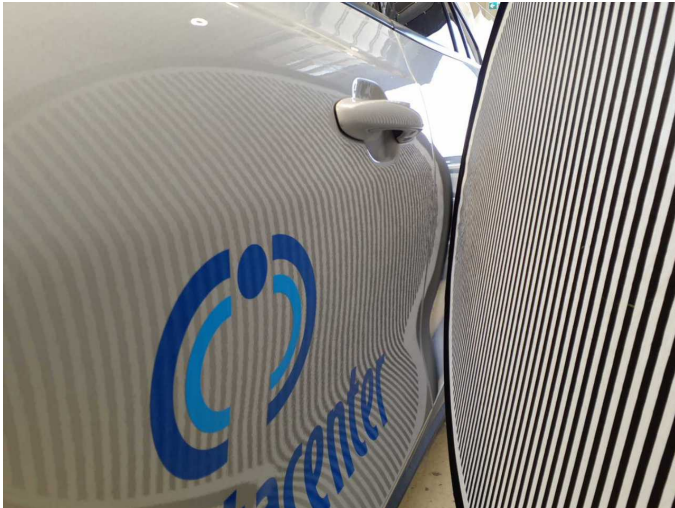
Damage 7: Door - front left side: Door (Wellig) - Unprofessionally repaired - Repair and paint
