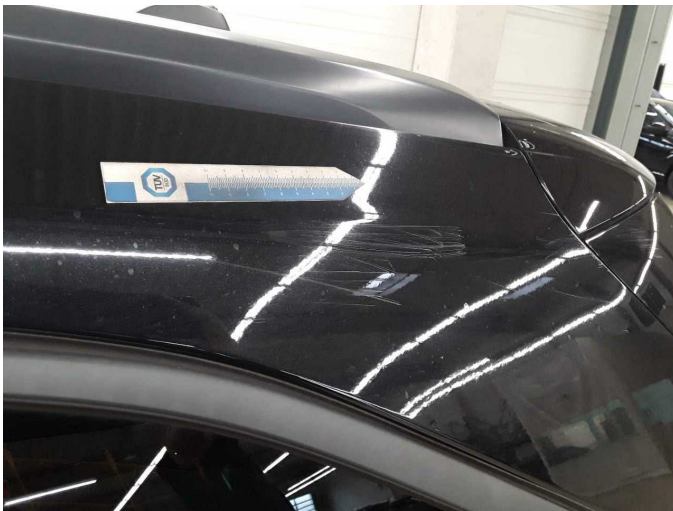
Damage 14: Side panel - rear left side: Side panel - Dent / paintcoat damage - Paint
