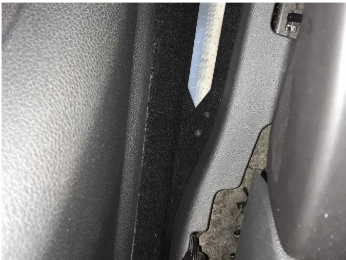
Damage 10: Trim / covers: Carpet - front left side - Burn hole (cigarettes) - Smart repair
