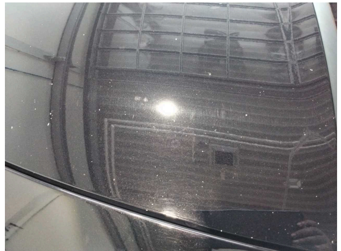
Damage 11: Bonnet: Bonnet - Stone chips - Paint
