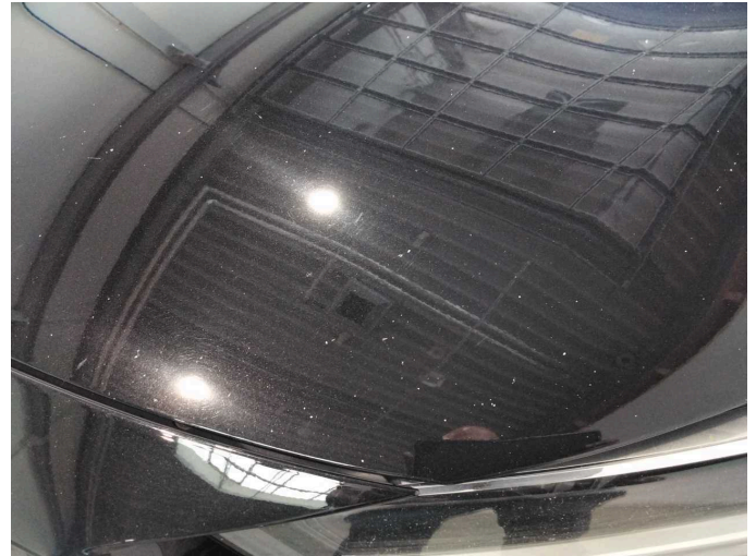
Damage 11: Bonnet: Bonnet - Stone chips - Paint
