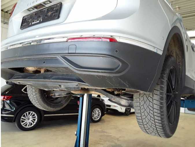
Damage 7: Rear bumper: Spoiler - Deformed - Replace
