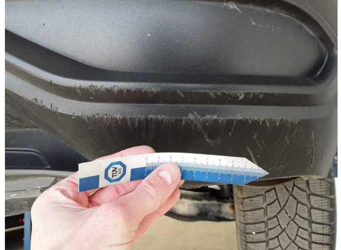
Damage 7: Rear bumper: Spoiler - Deformed - Replace
