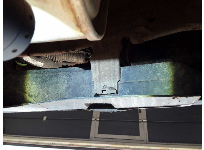
Damage 4: Rear bumper: Spoiler (Halter) - Deformed - Repair
