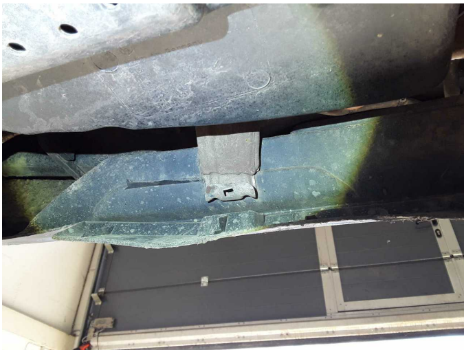
Damage 4: Rear bumper: Spoiler (Halter) - Deformed - Repair
