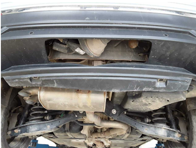
Damage 7: Rear bumper: Spoiler - Deformed - Replace
