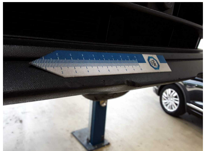
Damage 5: Front bumper: Spoiler - Scratched - Replace
