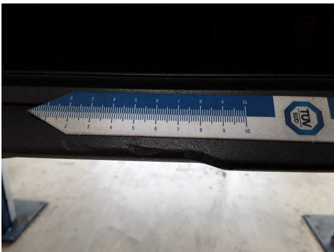
Damage 5: Front bumper: Spoiler - Scratched - Replace
