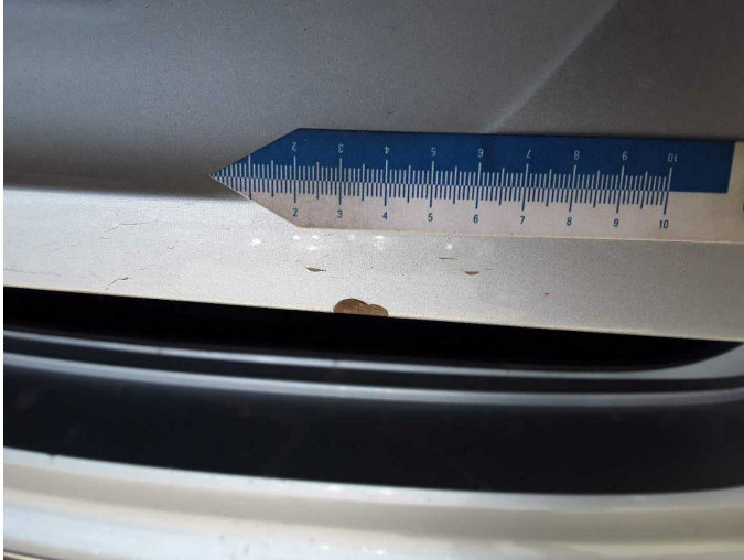
Damage 9: Boot lid / rear door: Boot lid (Blättert ab) - Corrosion - Repair and paint
