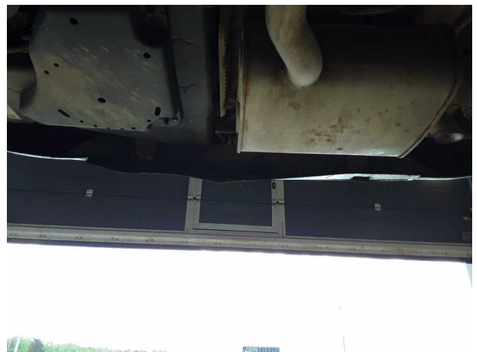
Damage 7: Rear bumper: Spoiler - Deformed - Replace
