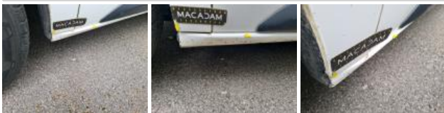
Side wall RL, Scratch(es), Paint
