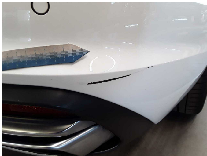
Damage 6: Rear bumper: Rear bumper - Scratch(es) - Paint
