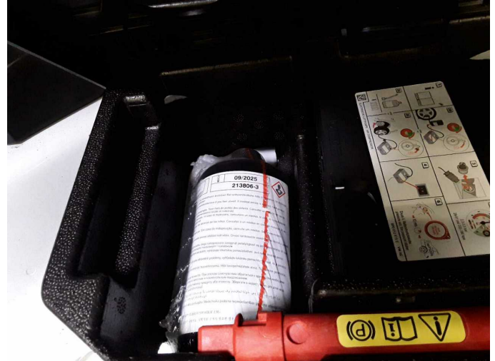
Damage 1: Equipment: Tirefit filler - Expired - Replace
