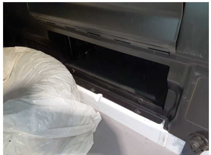
Damage 1: Trim / covers: Trim / covers - Missing - Replace
