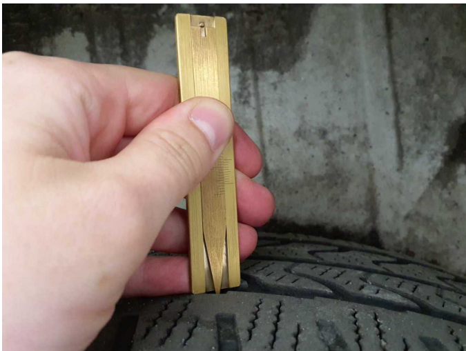
Damage 5: Wheel / tyres: Tyre - right (Winterreifen Profiltiefe <4mm) - Does not meet the leasing specifications - Replace
