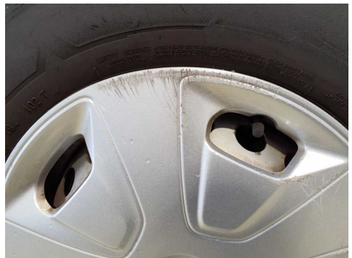
Wear and tear 6: Wheel / tyres: Wheel cover - front right side - Scratch(es) - No deduction
