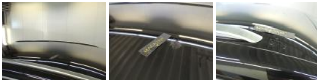
Roof, Chemical polution, Polish
