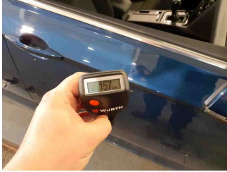
Paint thickness Door FR
