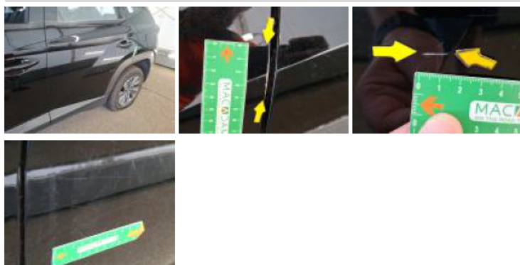
Aile ARG, Griffe(s), Acceptable
