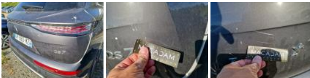
Fog light RL, Broken, Replace
