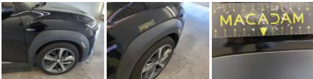
Wing RR, Scratch(es), Repair and paint (complete)
