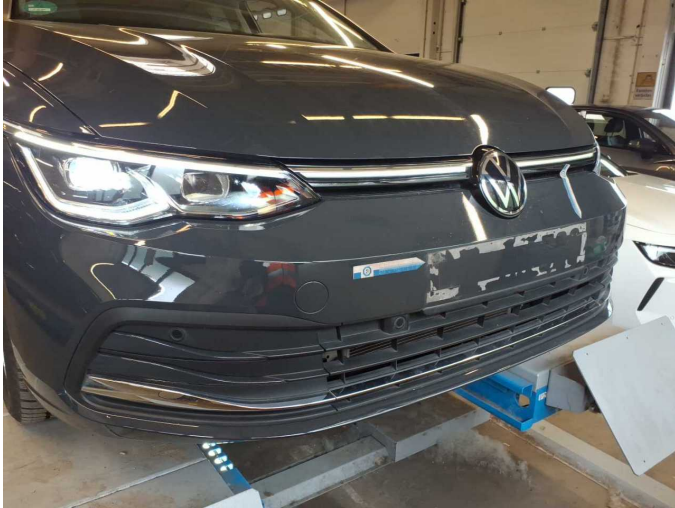
Damage 8: Front bumper: Front bumper (Beklebt) - Scratched - Paint
