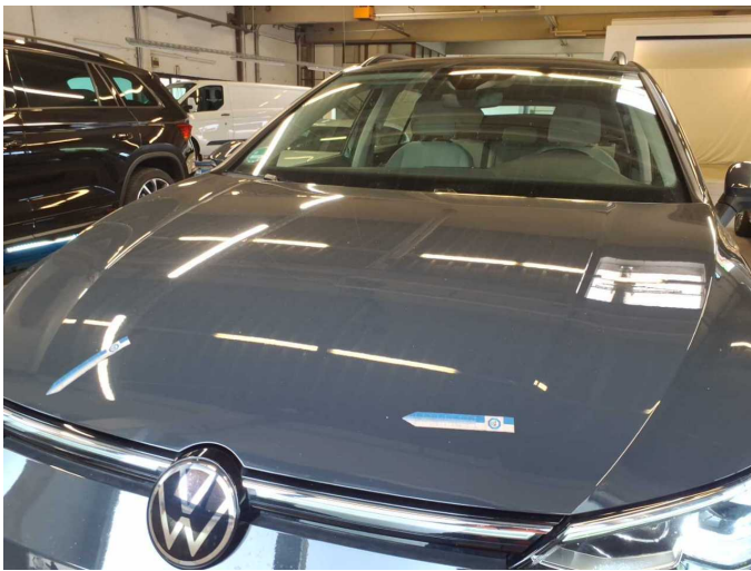
Damage 7: Bonnet: Bonnet - Dent / paintcoat damage - Repair and paint
