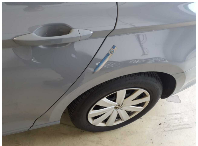
Damage 2: Side panel - rear left side: Side panel - dent(s) - Smooth repair work
