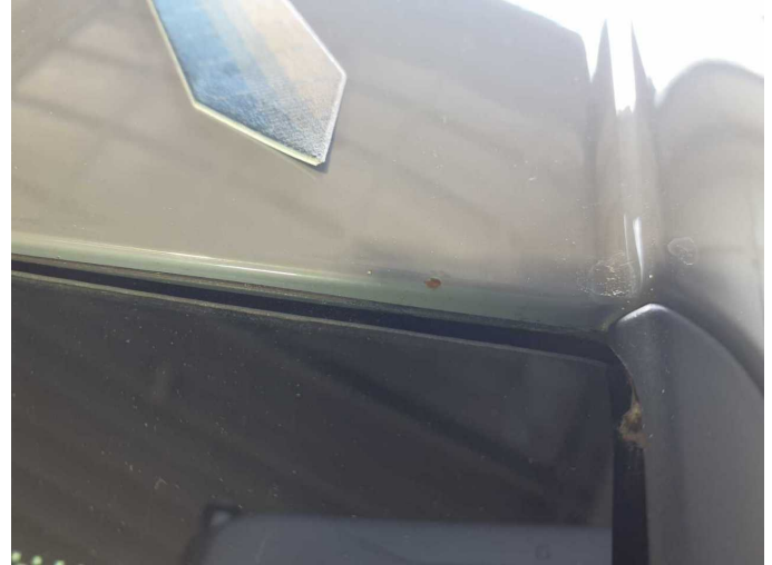
Damage 9: Roof: Roof - Stone chips - Smart repair
