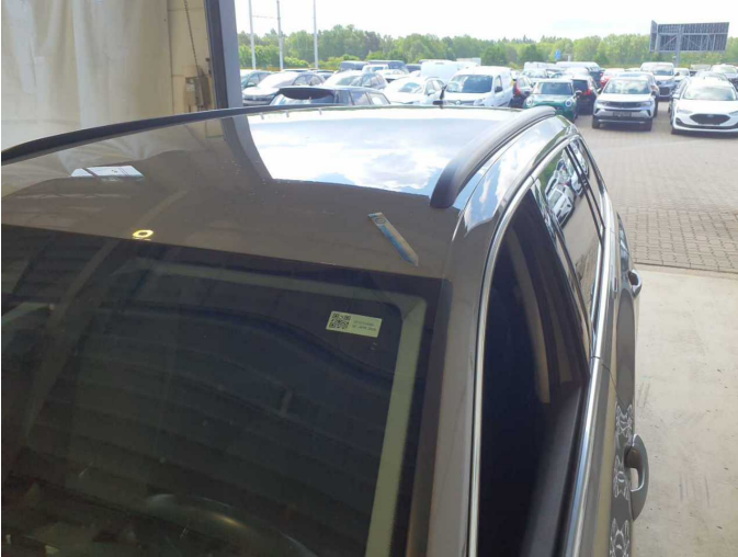
Damage 9: Roof: Roof - Stone chips - Smart repair
