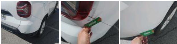
Reflector, Unclassped, Replace
