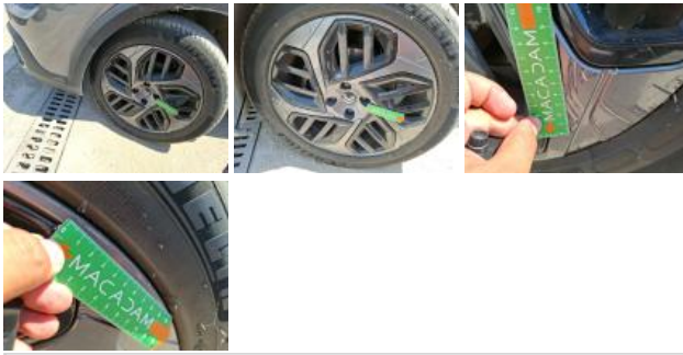
Tyre RL, Out of tolerance, Replace
