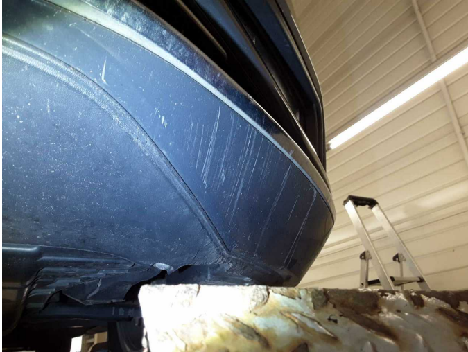
Damage 2: Front bumper: Front bumper - Scratch(es) - Paint
