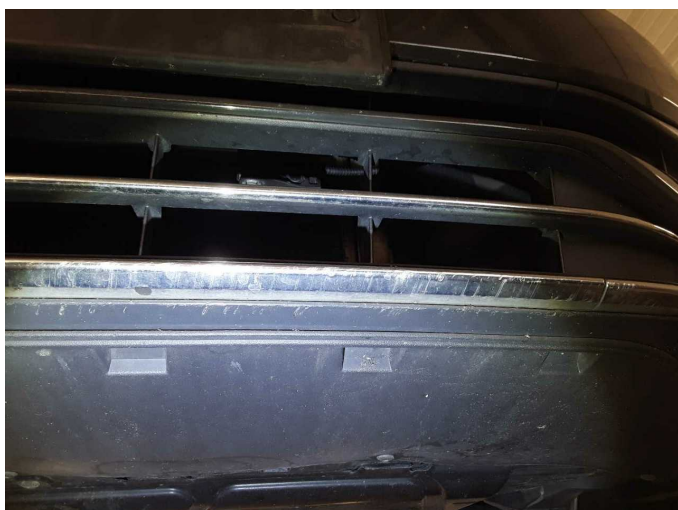
Damage 1: Trim / covers: Brightware / decorative strip (Stoßfänger vorn) - Scratched - Replace
