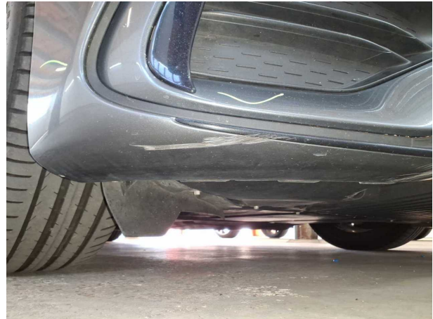
Damage #2: Front bumper: Front bumper - Scratched - Loss in value
