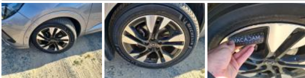
Tyre FL, Tear, Replace
