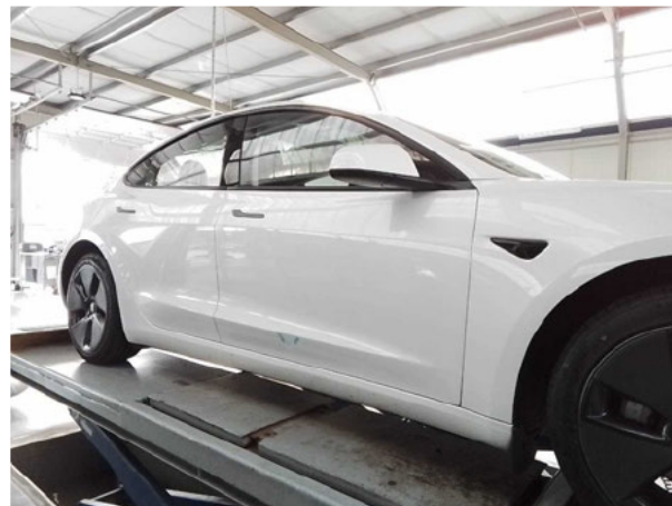
Beschädigung #2: Tür vorn rechts: Tür - Delle / Lackschaden - Smart Repair
