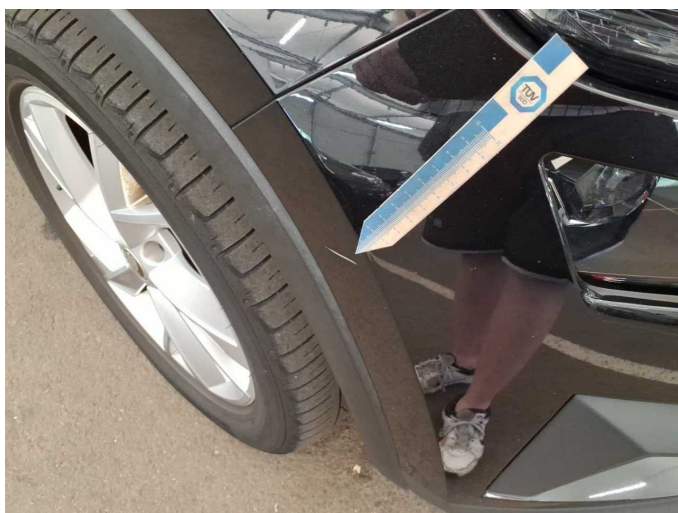
Damage 8: Front bumper: Front bumper - Scratched - Paint
