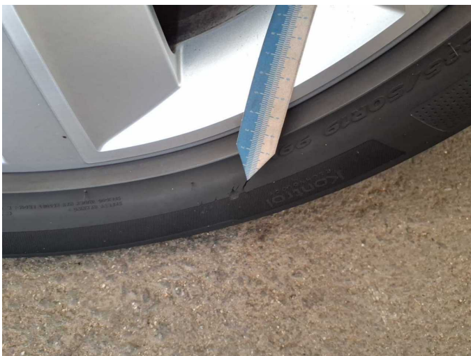
Damage 3: Wheel / tyres: Tyre - front left side - Broken / torn - Replace
