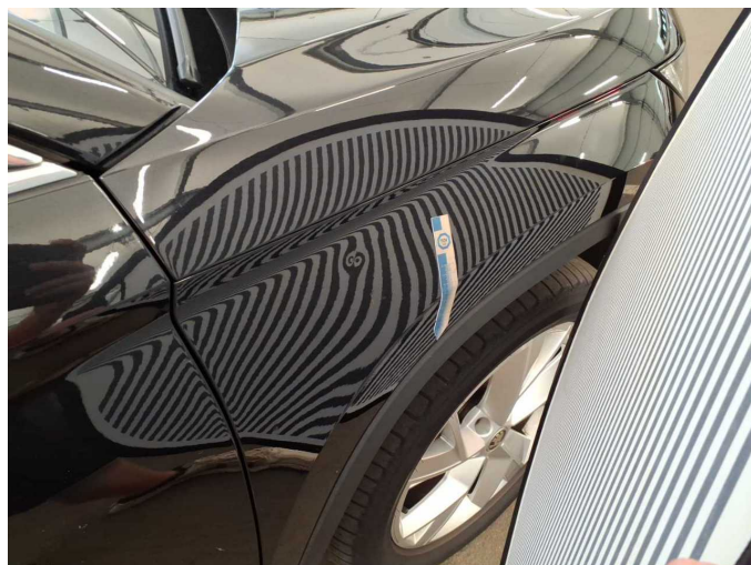
Damage 4: Mudguard - right side: Mudguard - right side - Dent / paintcoat damage - Repair and paint
