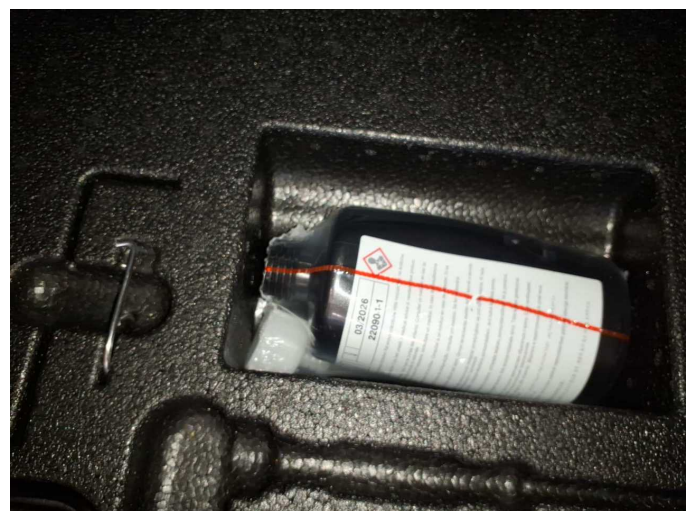
Damage 1: Equipment: Tirefit filler - Expired - Replace
