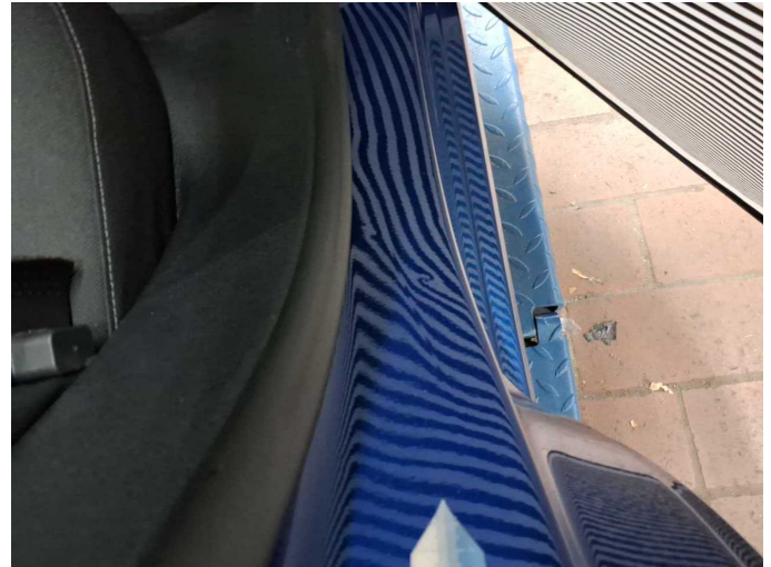
Damage 2: Side panel - rear right side: Sill - dent(s) - Smooth repair work
