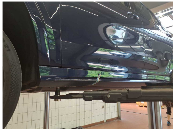
Wear and tear 1: Sill - left side: Trim (Unterhalb) - Dent / paintcoat damage - No deduction
