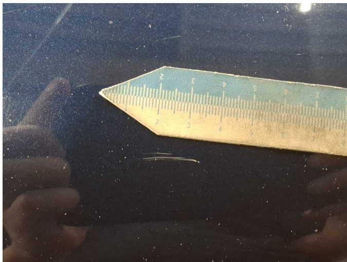
Damage 8: Bonnet: Bonnet (+ Kratzer) - Stone chips - Paint
