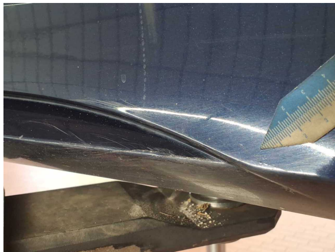
Damage 6: Sill - right side: Trim - Scratched - Paint
