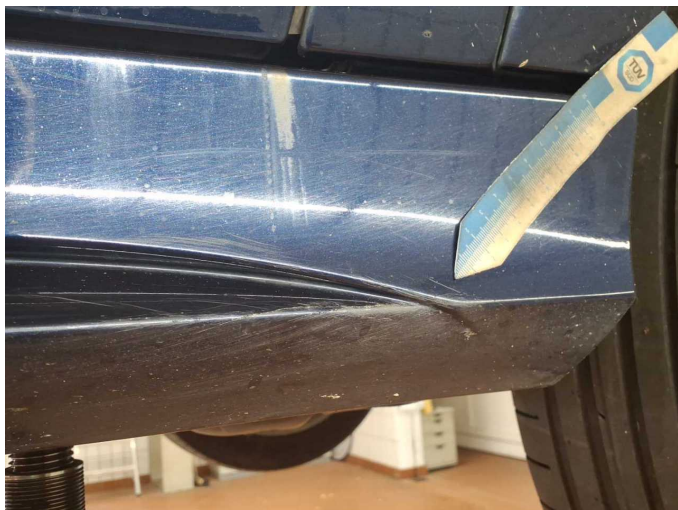
Damage 6: Sill - right side: Trim - Scratched - Paint
