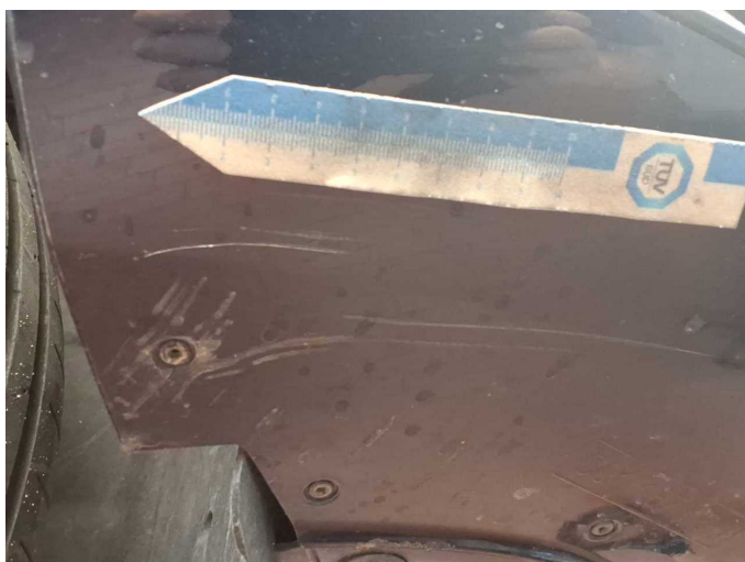
Damage 7: Front bumper: Front bumper (+ Steinschläge) - Scratch(es) - Paint
