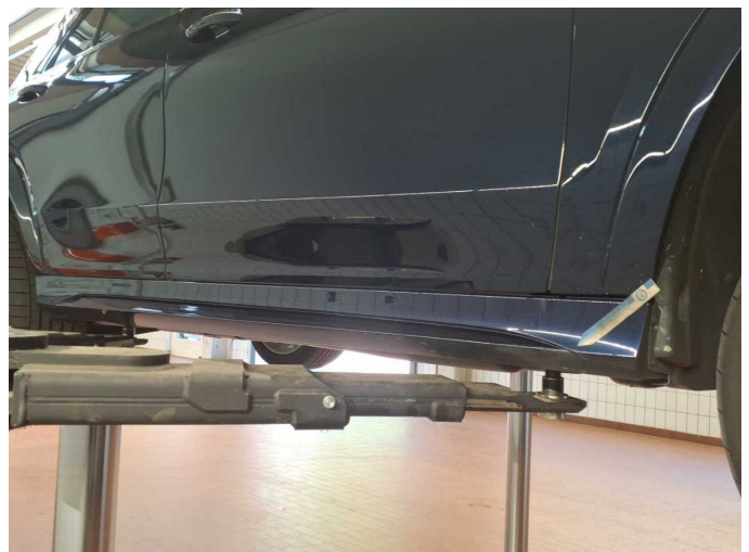
Damage 6: Sill - right side: Trim - Scratched - Paint
