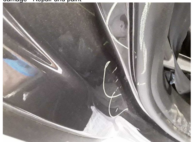
Damage #6: Side panel - rear right side: Sill - Dent / paintcoat damage - Repair and paint
