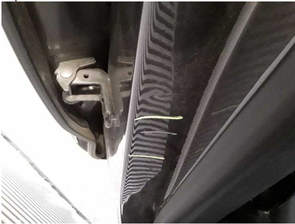
Damage #5: Sill - right side: Sill - Scratched - Repair and paint
