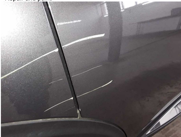
Damage #10: Door - rear right side: Door - Dent / paintcoat dama... - Repair and paint
