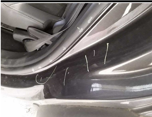
Damage #7: Side panel - rear left side: Sill - Dent / paintcoat damage - Repair and paint
