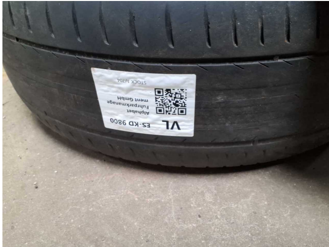
Damage 3: 2nd wheel set: 2 tyres - Worn - Replace
