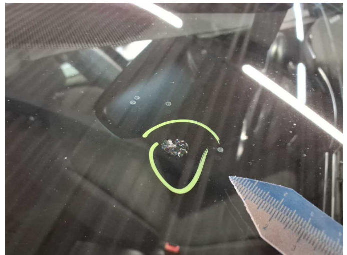
Damage 6: Vehicle glazing: Windscreen (Rissbildung) - Stone chips - repair according to calculation
