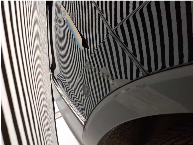
Damage 5: Rear bumper: Rear bumper (inkl. Radlauf) - Scratched - Paint
