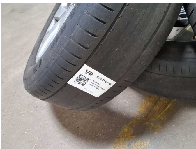
Damage 3: 2nd wheel set: 2 tyres - Worn - Replace
