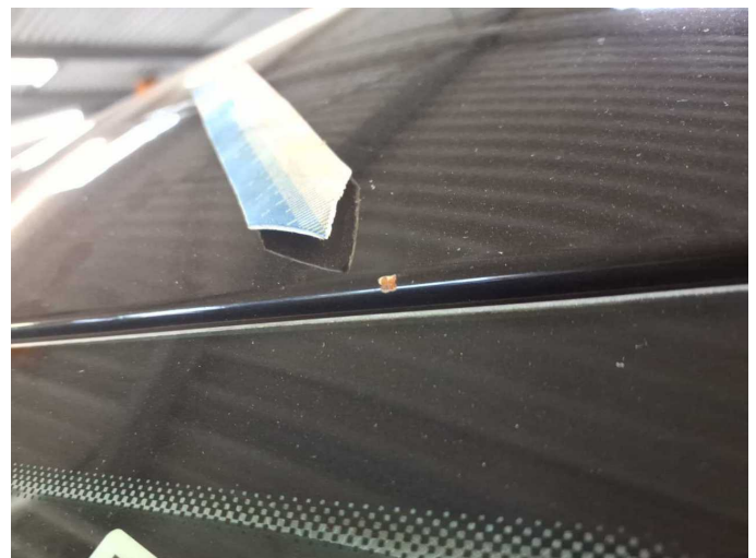
Damage 4: Roof: Roof - Corrosion - Smart repair
