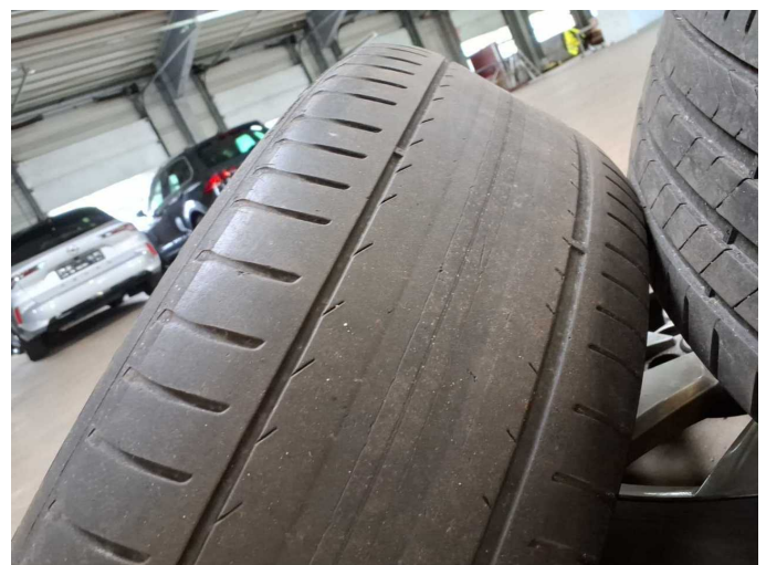
Damage 3: 2nd wheel set: 2 tyres - Worn - Replace
