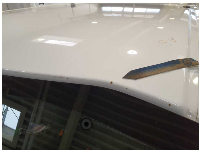
Damage 3: Roof: Roof - Corrosion - Smart repair
