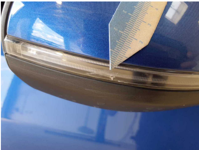
Damage 7: Indicator - front: Mirror - right side - Scratch(es) - Replace
