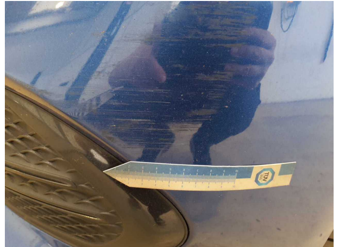
Damage 17: Front bumper: Front bumper - Scratch(es) - Paint
