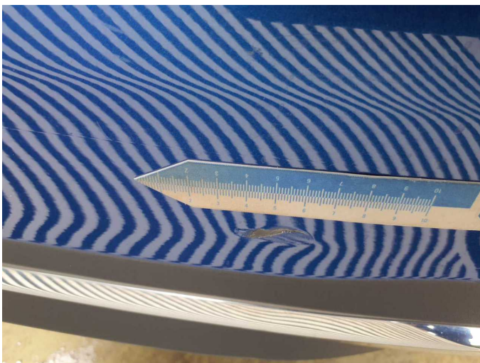
Damage 15: Rear bumper: Rear bumper - Dent / paintcoat damage - Repair and paint
