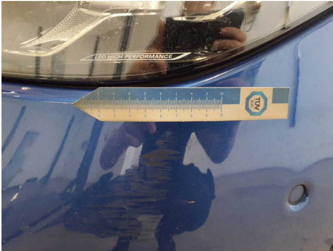
Damage 17: Front bumper: Front bumper - Scratch(es) - Paint
