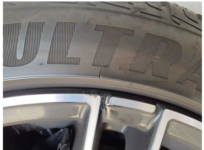
Damage 9: 2nd wheel set: 2 tyres - Porous / cracked - Replace
