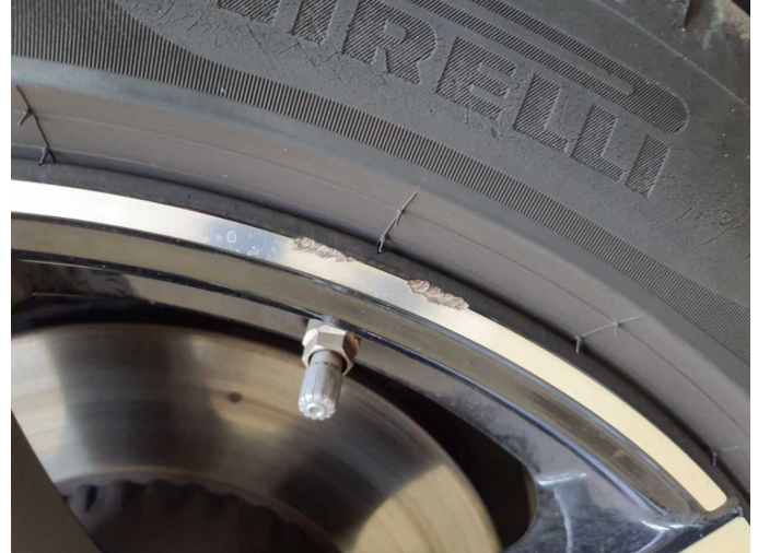
Damage 11: Wheel / tyres: Alloy rim - front right side - Scratch(es) - Replace
