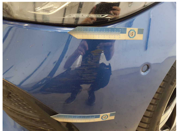
Damage 17: Front bumper: Front bumper - Scratch(es) - Paint
