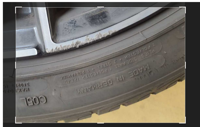
Damage 9: 2nd wheel set: 2 tyres - Porous / cracked - Replace
