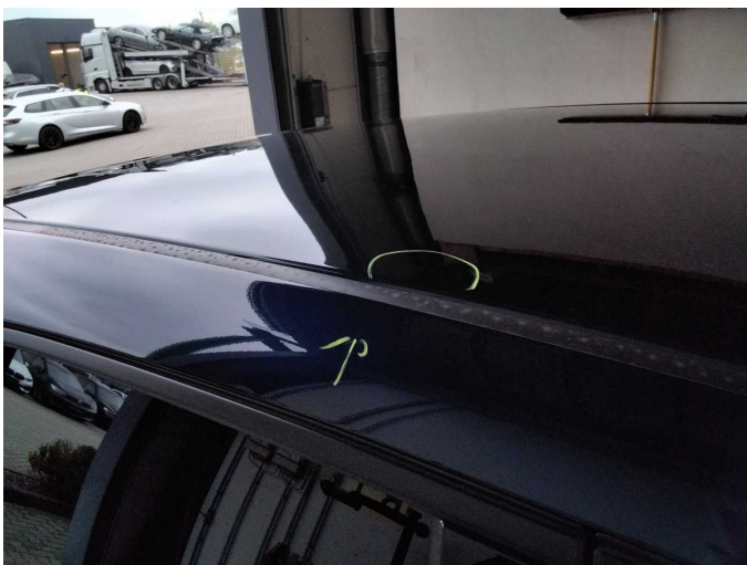
Damage 3: Roof: Roof - dent(s) - Smooth repair work
