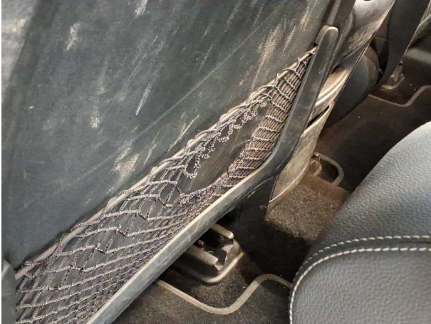
Damage #3: Interior: Separation net - Damaged - Replace
