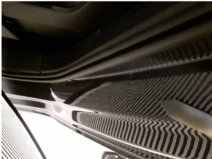
Damage 2: Body: C-pillar - left side - dent(s) - Smart repair
