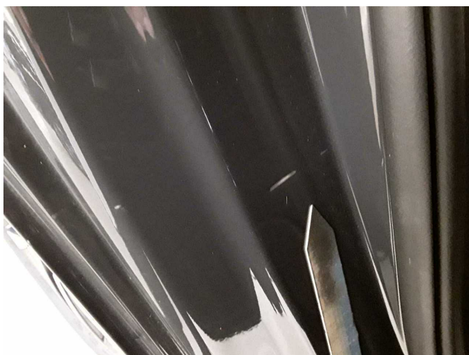
Damage 3: Body: C-pillar - right side - Scratch(es) - Smart repair
