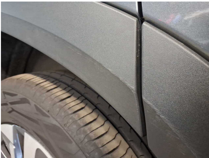
Damage 7: Side panel - rear right side: Wheel well extension (+ Türe HR) - Scratched - Replace
