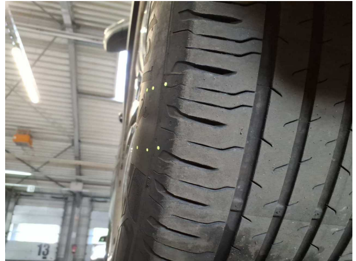
Wear and tear 5: Wheel / tyres: Tyre - front right side (produktionsbedingt) - Deformed - No deduction
