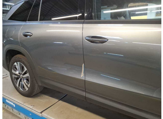
Damage 3: Door - rear right side: Door edge - Scratch(es) - Smart repair
