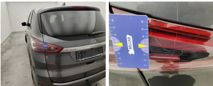
Light / Rear Left On Rear Bonnet / Replace-scratch
