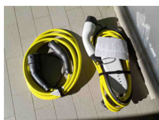
Charging cable (normal)
