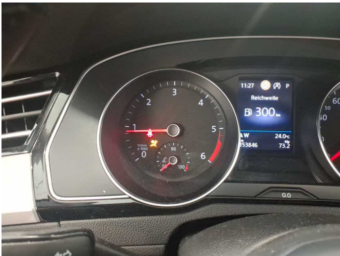
Damage 2: Instrument panel: Indicator light (Airbag Kontrollleuchte) - on - Perform diagnosis
