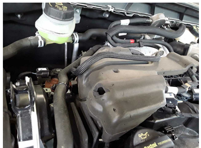
Damage 1: Engine: Engine cover (Isolierung) - Damaged - Replace
