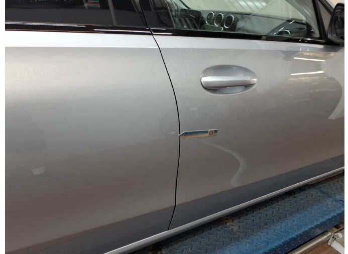
Damage 5: Door - rear right side: Door (Polieren) - Abrasion - Smart repair
