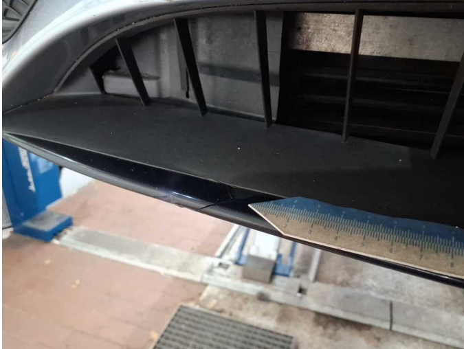
Damage 7: Front bumper: Spoiler (Lippe) - Broken / torn - Replace
