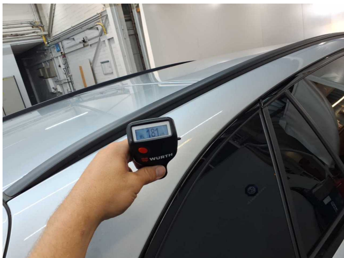
Repainting 1: Roof rail - right side, Mudguard - right side, Side panel - rear right side
