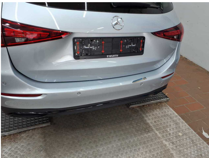
Damage 9: Rear bumper: Rear bumper - Scratch(es) - Paint
