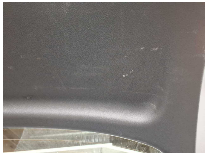
Damage 3: Trim / covers: Boot lid - interior trim - Scratch(es) - Loss in value
