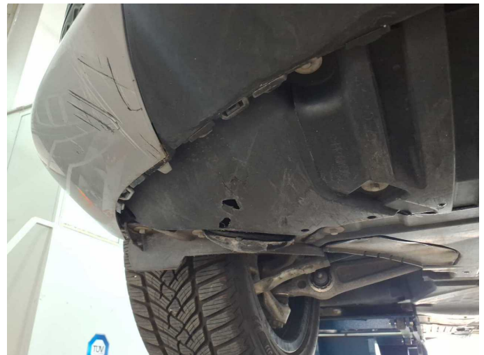
Damage 6: Body: Underbody panelling (Rechts) - Broken / torn - Replace
