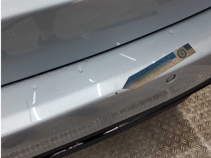
Damage 9: Rear bumper: Rear bumper - Scratch(es) - Paint
