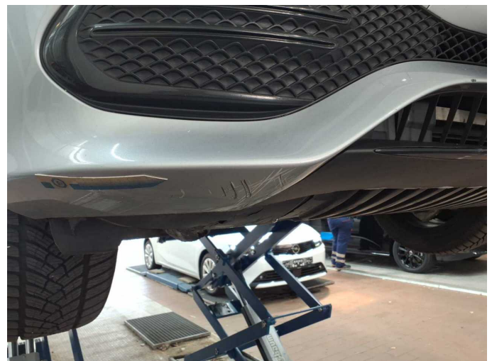
Damage 10: Front bumper: Front bumper - Scratch(es) - Paint
