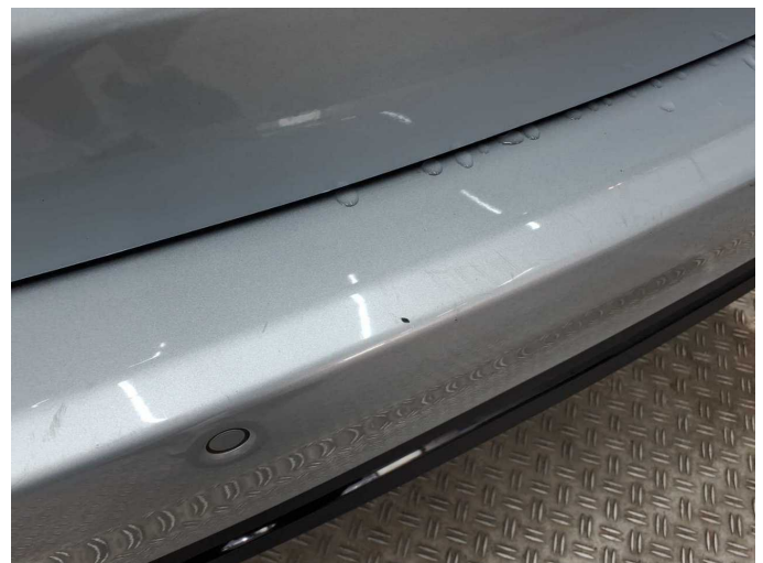
Damage 9: Rear bumper: Rear bumper - Scratch(es) - Paint
