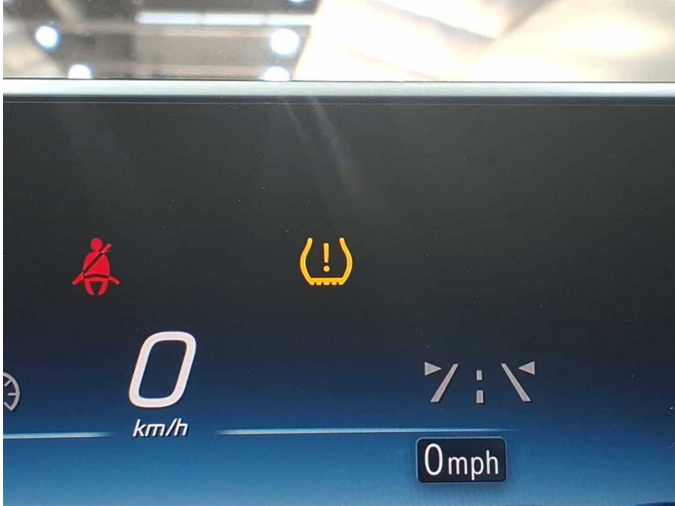
Damage 4: Instrument panel: Indicator light (Reifendruckkontrollsystem) - on - Perform diagnosis
