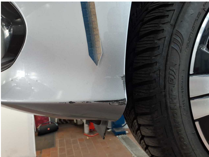
Damage 10: Front bumper: Front bumper - Scratch(es) - Paint
