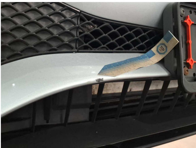
Damage 10: Front bumper: Front bumper - Scratch(es) - Paint
