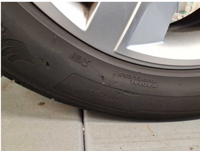
Damage 3: Wheel / tyres: Tyre - front right side (nicht fahrbereit) - Damaged - Replace
