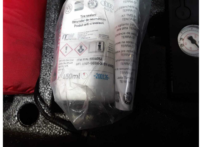
Damage 2: Equipment: Tirefit filler - Expired - Replace
