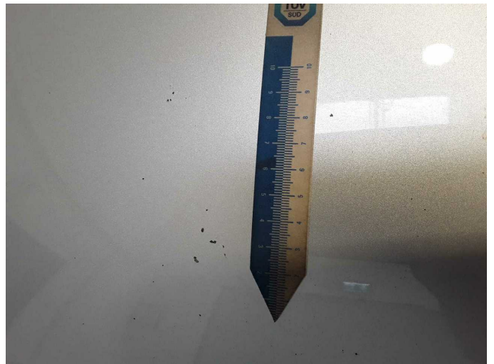
Damage 5: Bonnet: Bonnet - Stone chips - Paint
