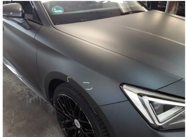
Damage #11: Mudguard - right side: Mudguard - right side - Scratch(es) - Paint
