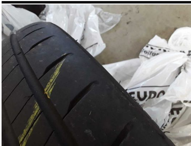
Damage #8: 2nd wheel set: 2 tyres - Worn - Replace
