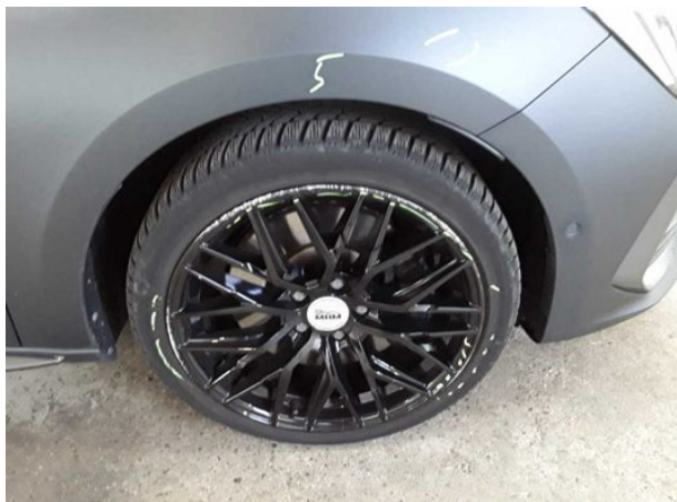
Damage #1: Wheel / tyres: Alloy rim - front right side - Scratched
