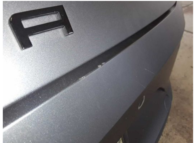
Damage #13: Rear bumper: Rear bumper - Scratch(es) - Paint
