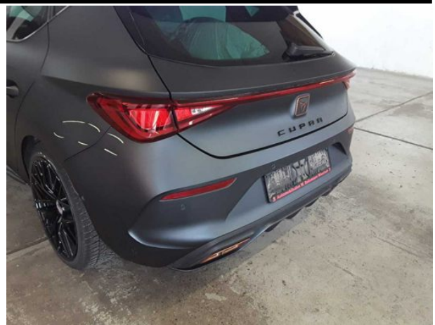
Damage #13: Rear bumper: Rear bumper - Scratch(es) - Paint
