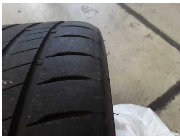
Damage #8: 2nd wheel set: 2 tyres - Worn - Replace
