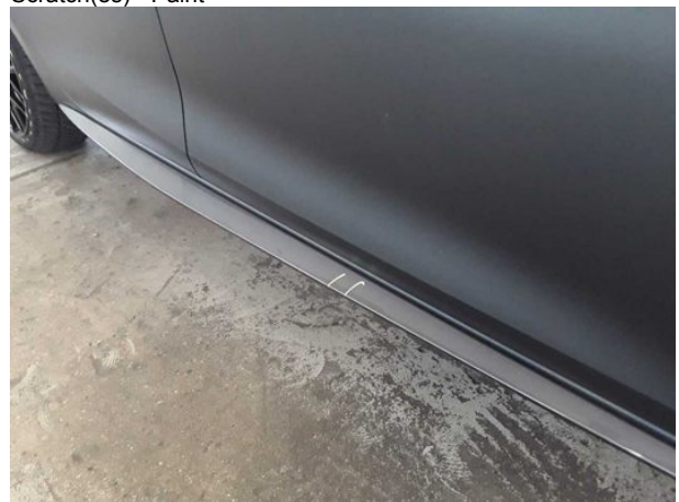
Damage #12: Sill - right side: Sill - Scratch(es) - Paint
