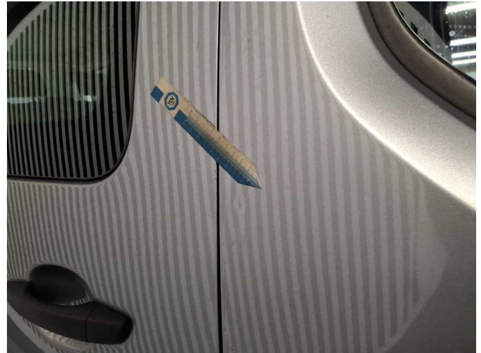
Damage 15: Door - front right side: Door - Dent / paintcoat damage - Repair and paint
