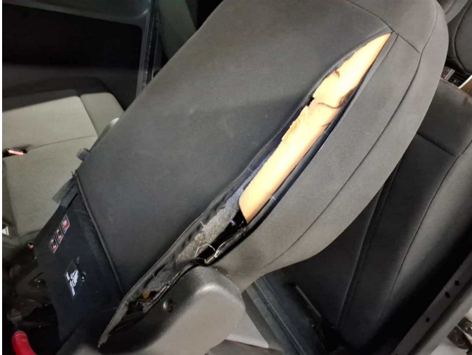
Damage 12: Seat - rear: Seat cover - 2nd row (Lehnenbezug) - Damaged - Replace
