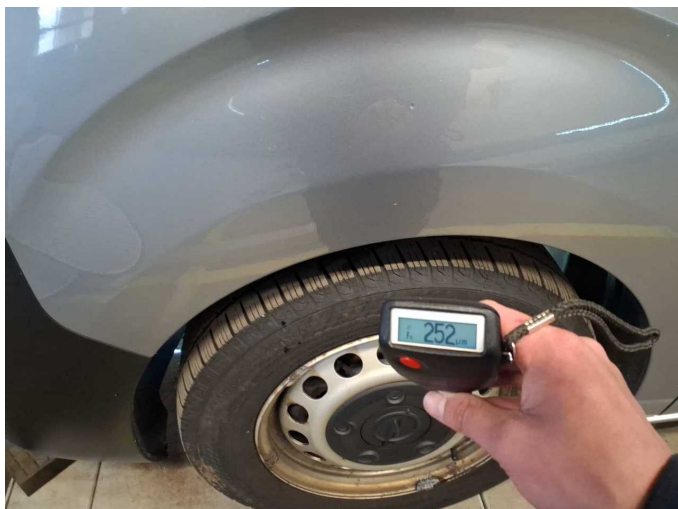
Repainting 1: Mudguard - left side
