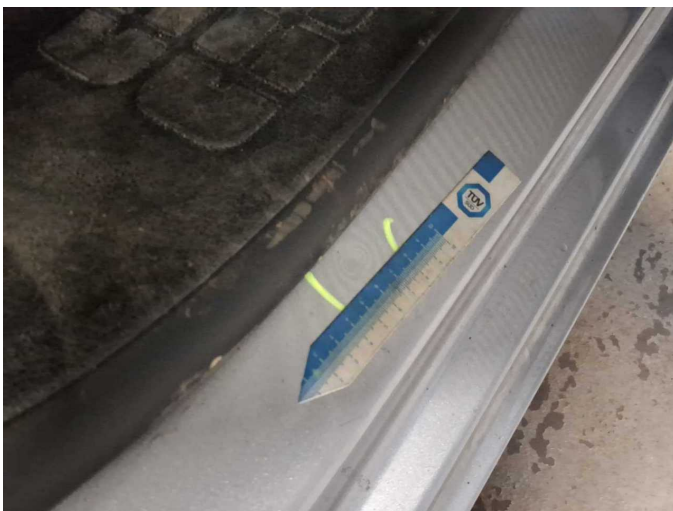
Damage 3: Sill - right side: Sill - dent(s) - Smooth repair work
