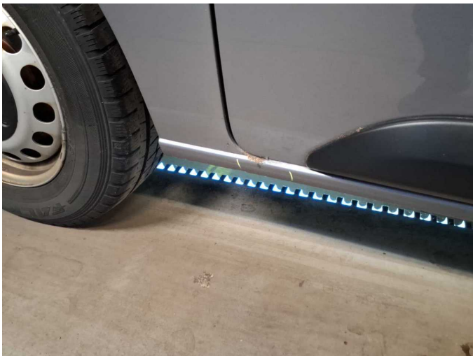
Damage 9: Sill - right side: Sill - Corrosion - Paint
