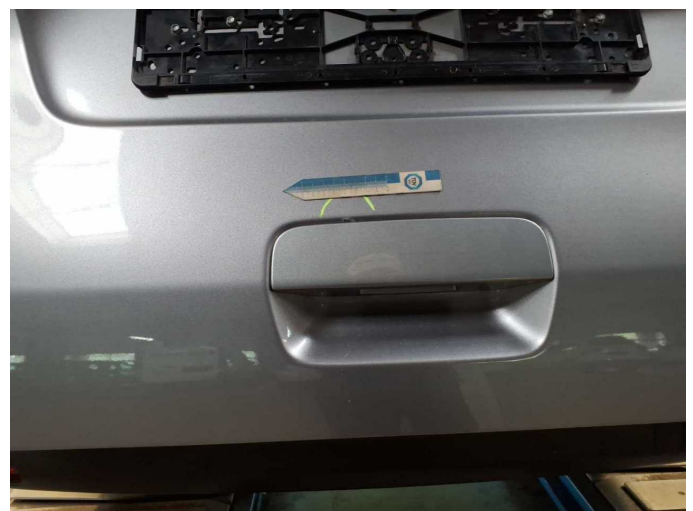
Damage 16: Boot lid / rear door: Boot lid - Dent / paintcoat damage - Paint
