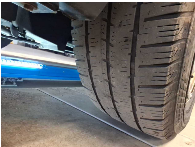
Damage 10: Wheel / tyres: Tyre - front - Does not meet the leasing specifications - Replace
