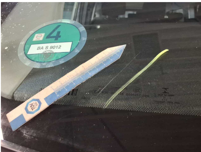
Damage 13: Vehicle glazing: Windscreen - Scratch(es) - Replace
