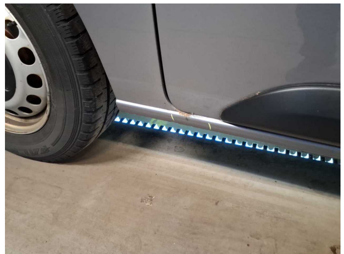
Damage 14: Sliding door, right: Sliding door (+Kratzer) - Corrosion - Paint
