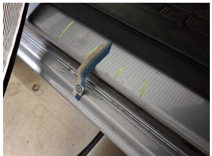
Damage 4: Side panel - rear right side: Side panel - dent(s) - Smooth repair work
