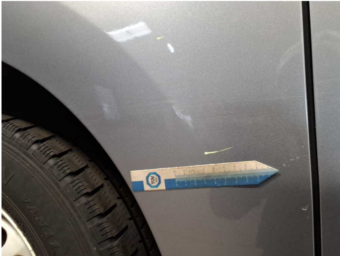
Damage 17: Side panel - rear right side: Side panel - Dent / paintcoat damage - Repair and paint
