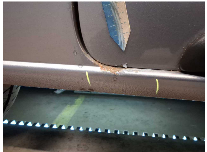
Damage 9: Sill - right side: Sill - Corrosion - Paint
