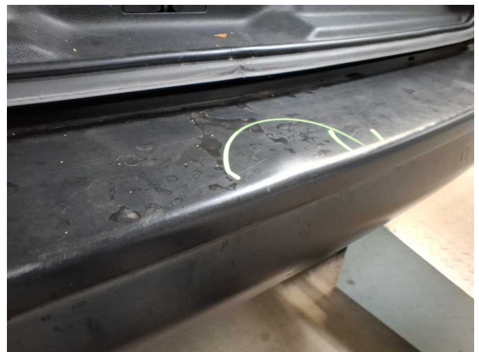
Damage 8: Rear bumper: Rear bumper (unpainted) - Deformed - Loss in value
